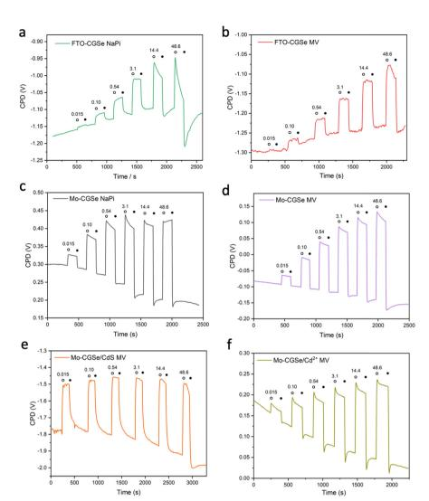
Fig. 5 Surface photovoltage (SPV) data as a function of light intensity (mW cm<sup>-2</sup>) from a 400 nm LED. (a) FTO-CGSe/NaPi, (b) FTO-CGSe/MV, (c) Mo-CGSe/NaPi, (d) Mo-CGSe/MV, (e) Mo-CGSe/CdS/MV, and (f) Mo-CGSe/Cd<sup>2+</sup>/MV
