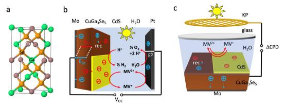
Fig. 1 (a) Crystal structure of  $CuGaSe_2$ , the parent phase of  $CuGa_3Se_5$ , (b) PEC cell, (c) liquid SPV configuration. MV = methylviologen.
