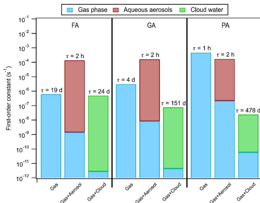
Fig. 7 Calculated first-order rate constants and corresponding lifetimes of FA, GA, and PA against  $\cdot\text{OH}$  (FA and GA) and direct photolysis (PA) in the atmosphere. The blue portions in the gas + aerosol conditions and gas + cloud conditions represent the contributions from gas phase reactions. The y axis is presented in a logarithm scale to accommodate the drastically different first-order constants.
