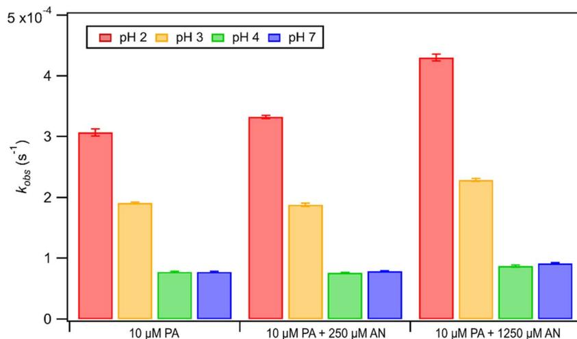
Fig. 6  $k_{\text{obs}}$  of PA at pH 2, 3, 4, and 7. The PA concentration was fixed at 10  $\mu\text{M}$ , while either 0  $\mu\text{M}$  or 250  $\mu\text{M}$  or 1250  $\mu\text{M}$  AN were used in these experiments. Error bars indicate the standard deviation of multiple experiments.
