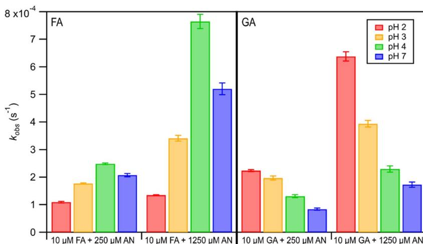
Fig. 3  $k_{\text{obs}}$  of FA and GA at pH 2, 3, 4, and 7. The concentrations of FA and GA were fixed at 10  $\mu\text{M}$ , while either 250  $\mu\text{M}$  or 1250  $\mu\text{M}$  AN were used in these experiments. Error bars indicate standard deviation of multiple experiments.
