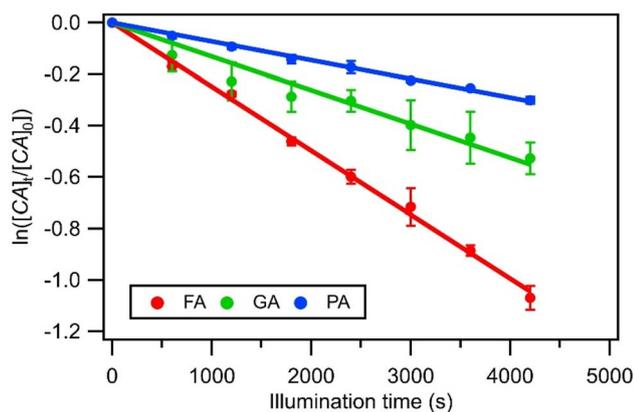
Fig. 2 Photodegradations of FA, GA, and PA in nitrate-mediated photooxidation experiments using 250  $\mu\text{M}$  AN at pH 4. Error bars represent standard deviations of repeated measurements. Lines show the exponential fit to the photodegradation data.
