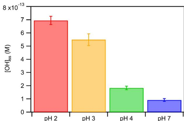
Fig. 4 Estimated  $[\cdot\text{OH}]_{\text{ss}}$  in nitrate-mediated photooxidation experiments using 250  $\mu\text{M}$  AN at pH 2, 3, 4, and 7. Error bars represent standard deviations of multiple experiments.
