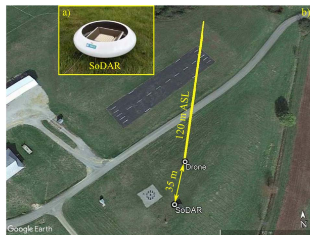
Fig. 4 (a) A close-up image of the SoDAR wind velocity profiler used to validate multirotor sUAS wind profiles. (b) A schematic of the experiment setup used at Virginia Tech Kentland Experimental Aerial Systems Laboratory on June, 29th, 2020 to validate multirotor sUAS wind velocity profiles next to SoDAR wind profiler.
