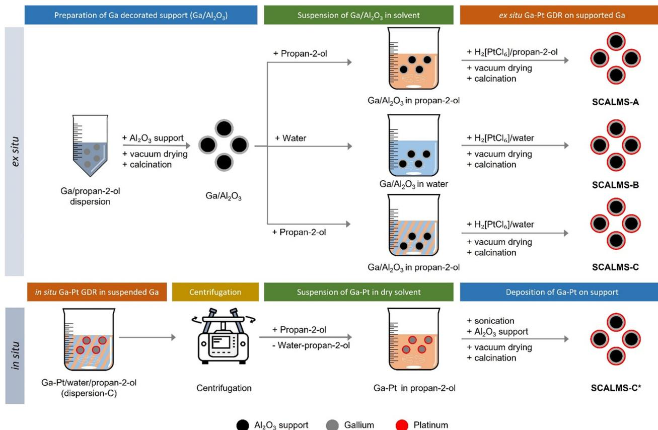
**Fig. 4** Preparation of different Ga-Pt SCALMS catalysts by *ex situ* galvanic displacement reaction in propan-2-ol, water, and water/propan-2-ol mixture. Ultrasonication of Ga is followed by deposition of the Ga droplets onto  $\text{Al}_2\text{O}_3$  support material. The galvanic displacement reaction between Ga-Pt happens on supported Ga droplets on  $\text{Al}_2\text{O}_3$ .
