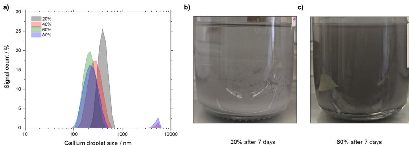
**Fig. 5** a) Particle size distribution of Ga droplets obtained from ultrasonication of Ga in propan-2-ol at different sonication amplitudes (20%, 40%, 60%, and 80%). Sonication time was 120 min in all cases. b) Photograph of the Ga dispersion at 20% amplitude after 7 days. c) Photograph of the Ga dispersion at 60% amplitude after 7 days.
