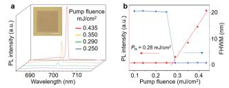
Fig. 3 (a) PL spectra of the BIPS@PMMA film-covered Ag nanoparticle array at different pump fluences. Inset: Bright-field microscopy image of the fabricated device. Scale bar is 50 µm. (b) Emission intensity (red) and FWHM (blue) as a function of pump fluence.
