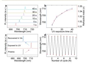
Fig. 4 (a) Time-dependent lasing spectra of the BIPS@PMMA filmcovered Ag nanoparticle array on exposure to UV light. (b) Plots of the lasing wavelength and refractive index of the BIPS@PMMA film-covered  $\mbox{\sc Ag}$ nanoparticle array versus time of exposure to UV light. (c) Lasing spectra of the BIPS@PMMA film-covered Ag nanoparticle array under alternate irradiation with UV and Vis light. (d) Plot of the lasing wavelength versus switching cycles.
