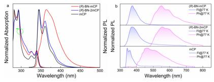
Fig. 2 (a) UV-vis spectra and PL spectra ( $\lambda_{ex}$  = 300 nm) measured in toluene solution (10<sup>-5</sup> M); (b) fluorescence and phosphorescence in the doped PMMA film (10%) at 77 K temperature ( $\lambda_{ex}$  = 300 nm).
