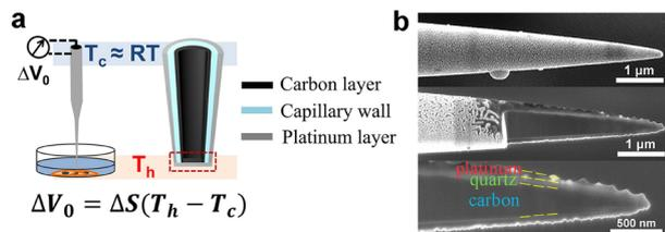
**Fig. 1** (a) Schematic diagram of a nanothermocouple probe for intracellular temperature sensing. (b) Side-view SEM images of the nanothermocouple probe (i) before and (ii) after FIB cutting; (iii) an enlarged view of the tip region in (ii).
