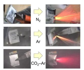
Fig. 1 Photographs of fully-charged small LIBs cut with nippers in N<sub>2</sub>, Ar, or CO<sub>2</sub>-Ar atmosphere.
