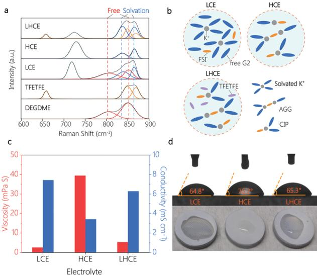
**Fig. 2** (a) Raman spectra of LCE, HCE and LHCE. (b) Schematic illustration of the solvation structure of LCE, HCE and the diluted LHCE. (c) Viscosity and ionic conductivity of LCE, HCE and LHCE. (d) Contact angles and wettability tests between the separator and different electrolytes.
