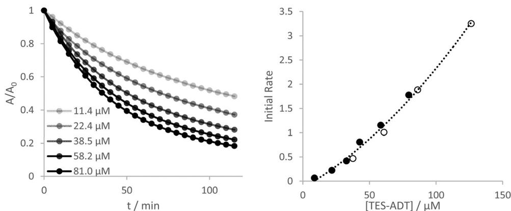
Fig. 4 Normalised absorption at 555 nm over time of solutions of TES-ADT in  $\text{CHCl}_3$  at different concentrations (darker = more concentrated) under illumination by green LED. (right) Plot of initial rate *versus* initial concentration. Filled circles monitored the first vibronic peak (555 nm) while the open circles were from a repeat experiment using the second vibronic peak (515 nm) allowing higher concentrations without saturating the detector.
