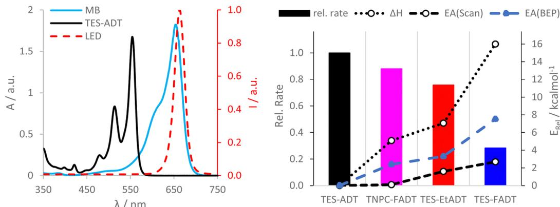
Fig. 6 Photosensitised oxidation of ADT derivatives using methylene blue in  $\text{CHCl}_3$ . (left) Absorption spectra of TES-ADT and methylene blue, and intensity spectrum of red LED. (bottom) Relative rate of endoperoxide formation of ADT derivatives (*versus* TES-ADT, left axis) and relative computed thermodynamic parameters (reaction enthalpy and activation energy *versus* TES-ADT, right axis).
