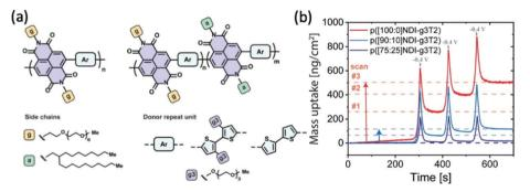
Fig. 13 (a) The chemical structures of D–A type **p(NDI-T2)** and **p(NDI-g3T2)** with alternating hydrophilic and hydrophobic side chains on the acceptor monomers. (b) The mass uptake changes of the series of NDI polymers with the increasing percentage of hydrophobic alkyl side chains. Reproduced from ref. 84 with permission from the American Chemical Society.
