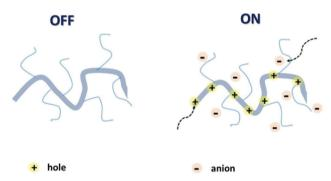
Fig. 2 Schematic representation of an OMIEC acting as a channel material in an accumulation mode OECT. Reproduced from ref. 30 with permission from Springer Nature.
