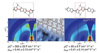
Sections of chemical structures of pgBTTT and p(g2T-TT) addressing S-O interactions with corresponding GIWAXS maps. Reproduced from ref. 78 with permission from the American Chemical Society.
