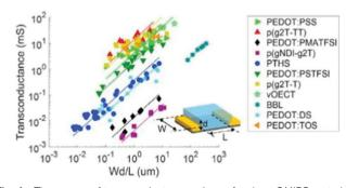
Fig. 4 The ranges of transconductance values of various OMIEC materials. The dotted lines correspond to the best fits of transconductance  $g_{\rm m} = \alpha W d/L$ , with  $\alpha$  being a proportionality constant.<sup>42</sup> Reproduced from ref. 44.
