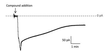
Fig. 6 Sample current recording after Na[o-FESAN] addition to the feeding side of the chamber. The stripping side was electrically grounded. Negative current implies that the [o-FESAN] anion crosses the membrane
