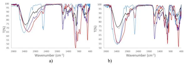
Fig. 3 (a) IR spectra of 2 mM Na[o-FESAN] in aqueous solution (blue), in DMEM (without phenol red) (red), and in DMEM + 10% FBS (purple). (b) IR spectra of 2 mM Na[8,8'-l2-o-FESAN] in aqueous solution (blue), in DMEM (red), and in DMEM + 10% FBS (purple). As a control: IR spectra of DMEM (black) and DMEM + 10% FBS (grey).
