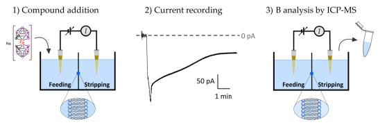
Fig. 2 Experimental method for the recording of compound-induced current in planar bilayers and determination of compound concentration in terms of the amount of boron by ICP-MS.
