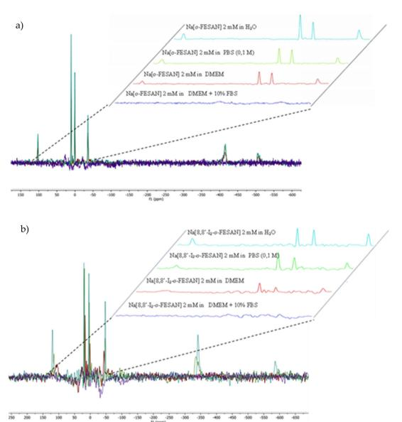
Fig. 4 (a) The  $^{11}$ B( $^{1}$ H}-NMR spectrum of 2 mM Na[o-FESAN] in aqueous solution (blue), in 0.1 M phosphate buffer (green), in DMEM (red), and in DMEM + 10% FBS (purple). (b)  $^{11}$ B( $^{1}$ H}-NMR spectrum of 2 mM Na[8,8'-I<sub>2</sub>-o-FESAN] in aqueous solution (blue), in 0.1 M phosphate buffer (green), in DMEM (red), and in DMEM + 10% FBS (purple).
