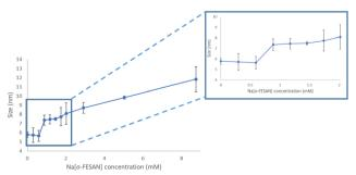
Fig. 5 Graphical representation of the hydrodynamic diameter (nm) of the DMEM + 10% FBS culture medium measured by DLS *versus* increasing concentrations of Na[o-FESAN] in water in the concentration range from 0 to 9 mM.
