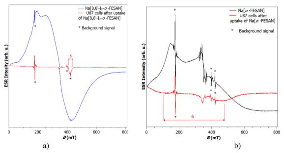
Fig. 1 (a) Spectra of Na[8,8'- $I_2$ -o-FESAN] in powder, U87 cells after uptake of Na[8,8'- $I_2$ -o-FESAN]. The g factor indicated by number 5 is 1.7. (b) Spectra of Na[o-FESAN] in powder and U87 cells after uptake of Na[o-FESAN]. The g factor indicated by number 6 is approximately 2.
