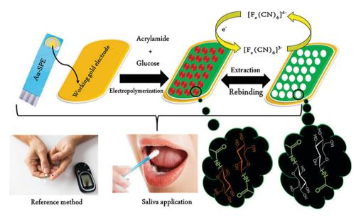
Fig. 8 Fabrication of a MIP-based screen-printed gold electrode (Au-SPE) for the diagnosis of diabetes mellitus prepared in the presence of glucose as the template, where the binding sites of molecular interactions have been highlighted. Traditional methods of finger-prick blood sampling have been presented as a comparison to emphasise the ease and pain-free means of saliva sampling. Reproduced with permission from ref. 196, Copyright 2019 Fisevier
