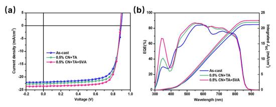
Fig. 2 (a) J-V curves and (b) EQE spectra and corresponding integrated  $J_{sc}$  of the PTQ10:Y26 devices with different treatments
