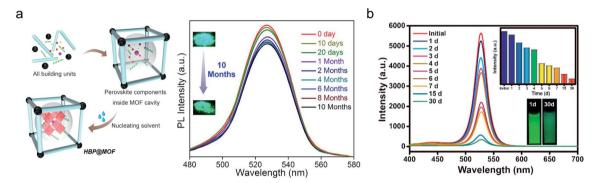
Fig. 5 Moisture stability of PeMOF. (a) PeMOF structures developed by Mollick et al., where the emission from the perovskite remains strong over 10 months of air exposure, Reprinted with permission from ref. 103, Copyright 2019 American Chemical Society, (b) Photoluminescence spectra of the PeMOF developed by Zhang et al., which exhibits robust emission when immersed in water for 30 days. Reprinted with permission from ref. 102. Copyright 2018 American Chemical Society.
