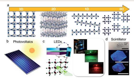
Fig. 1 (a) Schematic illustration of the metal halide perovskite structures in 3D, 2D, 1D and 0D. (b) Cartoon illustrations of a perovskite photovoltaic panel. (c) The typical device structure for a perovskite light-emitting diode and photos of perovskite LEDs with tunable colors. (d) Photos of a 2D perovskite crystal that lights up upon UV light (middle panel) and X-ray (lower panel) irradiation. Reproduced from ref. 11 with permission from Springer Nature.
