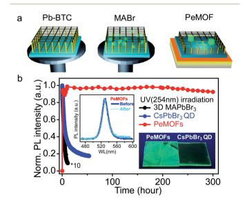
Fig. 9 (a) Illustration of the PeMOF thin film fabrication process via a two-step spin coating method. (b) Time evolution of the normalized photoluminescence intensities of the 3D MAPbBr<sub>3</sub> thin film, CsPbBr<sub>3</sub> QD thin film and PeMOF thin film. The PL spectrum for a PeMOF thin film before and after UV irradiation is plotted in the inset, and a photo of the PeMOF versus QD thin films after aging is shown in the same plot. Reproduced from ref. 20 with permission.
