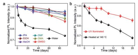
Fig. 6 The normalized PL intensity of the PeMOF fabricated by Mollick *et al.* tested in (a) various solvent systems and (b) over 20 days with heat stress and under constant UV illumination. Reprinted with permission from ref. 103. Copyright 2019 American Chemical Society.
