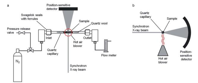
Fig. 17 Schematic of an experimental setup used to study pyrolysis of a gelatin/Fe(NO<sub>3</sub>)<sub>3</sub> mixture in situ viewed from (a) the top and (b) the side. Figure reproduced with permission from ref. 223.
