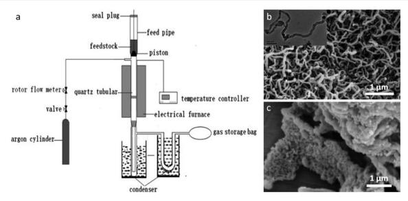
Fig. 12 (a) Diagram of setup for fast pyrolysis and SEM images of samples prepared by fast pyrolysis of sawdust powder with (b) FeCl<sub>3</sub> (inset TEM image) and c) Fe(NO<sub>3</sub>)<sub>3</sub>. Figures modified with permission from ref. 161 and 162.
