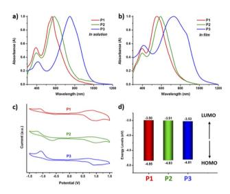
Fig. 5 Characterization of polymers P1, P2 and P3 (a) UV-vis absorption spectra in chloroform solution; (b) as a thin film. (c) cyclic voltammograms as a thin film (scan rate  $100~{\rm mV~s}^{-1}$ ) and (d) HOMO–LUMO energy level diagram obtained using CV measurement.
