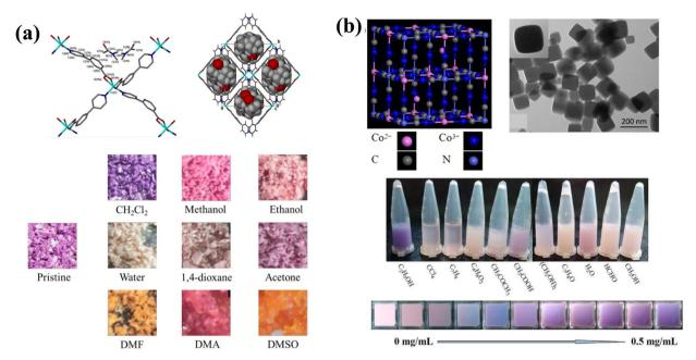
Fig. 3 (a) Coordination environment of Co(ii), packing of  $\{[Co(3,4pba)_2-(H_2O)]\cdot 1/2DMF\cdot H_2O\}_n$ ; and pictures of powdered samples after exposure to different solvents. Figures adapted from ref. 126. (b) Structure of  $Co_3[Co(CN)_6]_2$  and TEM image of the nanoparticles; the colour of  $Co_3[-Co(CN)_6]_2$  films changes from pink to purple gradually with an increasing ethanol concentration gradient. Adapted with permission from ref. 96.
