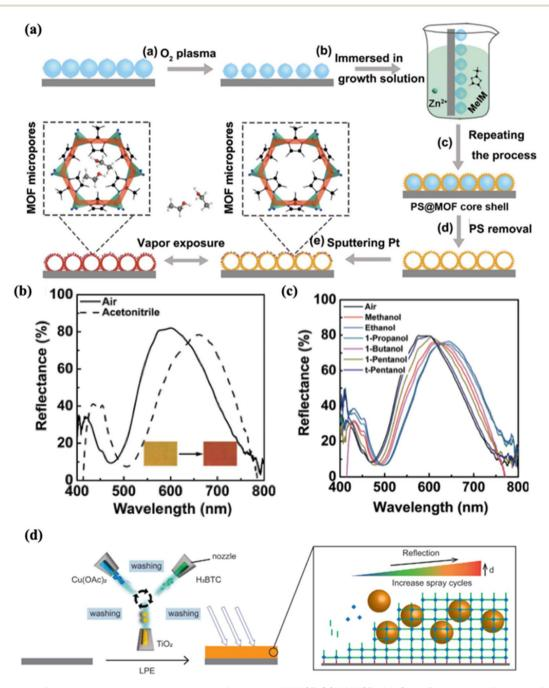
Fig. 9 (a) Illustration of the experimental procedure used to fabricate a HMNSE. (b) HMNSE with 2 nm Pt coating before and after exposure to saturated acetonitrile vapour at 293 K. The insets show the corresponding optical microphotographs. (c) Optical response of the HMNSE to different alcohols, including methanol, 1-propanol, 1-butanol, 1-pentanol, and tert-pentanol. (d) Schematic of the liquid phase epitaxy (LPE) method for sequential TiO<sub>2</sub>-loading in MOF films. (11)
