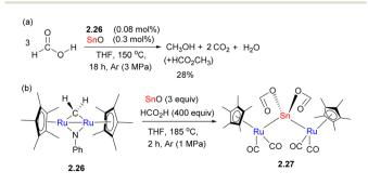
Scheme 13 Formic acid disproportionation to methanol catalyzed by Ru/Sn complex (a) and isolation of a trinuclear Ru-Sn-Ru complex (b).
