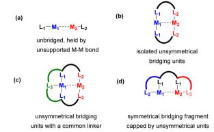
Scheme 2 Commonly used motifs for unsymmetrical ligand scaffold design in heterobi- or multimetallic complexes: (a) unbridged complexes supported by mononucleating ligands and held by metalmetal interactions; (b) complexes containing one or more isolated unsymmetrical bridging units; (c) complexes in which several bridging units are linked with a common linker; (d) heterobimetallic complexes containing a bridging fragment capped by unsymmetrical coordinating units.
