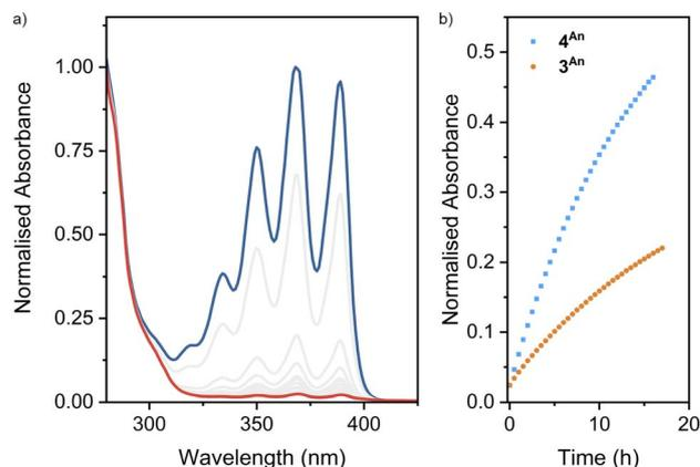
**Fig. 5** (a) Absorption spectra of **4<sup>An</sup>** ( $2.5 \times 10^{-4}$  M) in DMSO before (blue) and after (red) 15 min irradiation at 365 nm and (b) thermal cycloreversion ( $\lambda_{\text{abs}} = 389$  nm) of **3<sup>An</sup>** ( $5 \times 10^{-4}$  M) and **4<sup>An</sup>** ( $2.5 \times 10^{-4}$  M) at room temperature.
