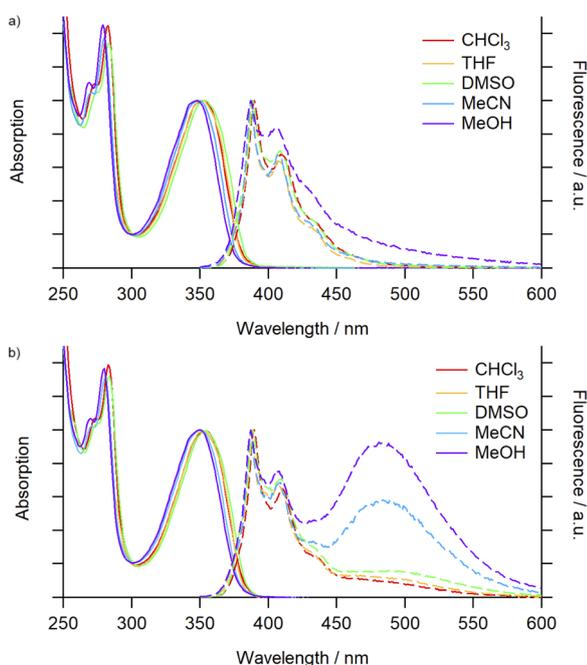
Fig. 1 Absorption (solid trace) and emission (dashed trace) spectra (air-equilibrated) of (a) **3<sup>Py</sup>** ( $5.2 \times 10^{-6}$  M) and (b) **4<sup>Py</sup>** ( $2.6 \times 10^{-6}$  M) in various solvents.
