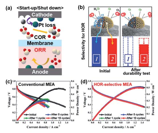
Fig. 3 (a) Schematic illustration of electrode reactions occurring under start-up/shut-down conditions. (b) Comparison of the oleylamine-attached Pt catalyst and carbon-encapsulated Pt catalyst for selective HOR. Changes in the single cell performance of the (c) conventional MEA and (d) HOR-selective MEA during start-up/shut-down cycles. Reproduced from ref. 41 with permission, copyright 2019, American Chemical Society.
