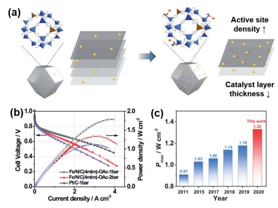
Fig. 7 (a) Schematic diagram of Fe-doping on ZIF-8 with acetates (OAC<sup>-</sup>). (b) Polarization and power density curves of Fe/N/C and Pt/C under  $H_2/O_2$  flow with 1 or 2 bar of backpressure. (c) Maximum power density ( $P_{max}$ ) of Fe-N-C catalysts in recent years. Reproduced from ref. 112 with permission, copyright 2021, Wiley-VCH.
