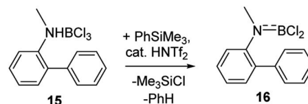
Scheme 6 Dehydrochlorination mediated by Me_3SiNTf_2 .
