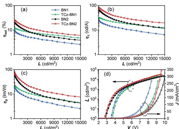
**Fig. 7** EL characteristics of OLED devices based on **BN1**, **TCz-BN1**, **BN2** and **TCz-BN2**. (a) The external quantum efficiency ( $\eta_{\text{ext}}$ ), (b) current efficiency ( $\eta_{\text{c}}$ ) and (c) power efficiency ( $\eta_{\text{p}}$ ) versus luminance ( $L$ ) curves for the devices; (d) luminance ( $L$ )–voltage ( $V$ )–current density ( $J$ ) characteristics for the devices.
