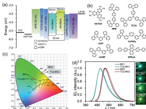
**Fig. 6** (a) Device structures and energy level diagrams of devices i and ii. (b) Molecular structures of the functional materials used in OLED devices. (c) The CIE 1931 chromaticity diagram and (d) EL spectra of devices recorded at  $1000 \text{ cd m}^{-2}$ . Photographs showing the emission colours of the device at a luminance  $\approx 1000 \text{ cd m}^{-2}$ .
