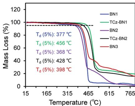
Fig. 1 Thermogravimetric curves of all the compounds.
