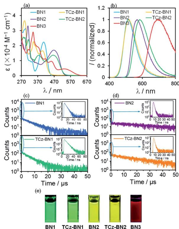
Fig. 5 (a) UV-Vis absorption spectra and (b) emission spectra (excitation at 406 nm, 398 nm, 465 nm, 464 nm and 531 nm for **BN1**, **TCz-BN1**, **BN2**, **TCz-BN2** and **BN3**, respectively) of all five compounds; (c and d) transient PL decay curves in THF solution under  $N_2$  conditions at 298 K; (e) photographs showing the emission colours of all five compounds.
