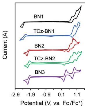
Fig. 4 Cyclic voltammograms (CV) for all compounds. The CV curves were measured at room temperature with 0.1 M solution of [*n*-Bu<sub>4</sub>N]PF<sub>6</sub> in dichloromethane for the oxidation and reduction scan (vs. Fc/Fc<sup>+</sup>).
