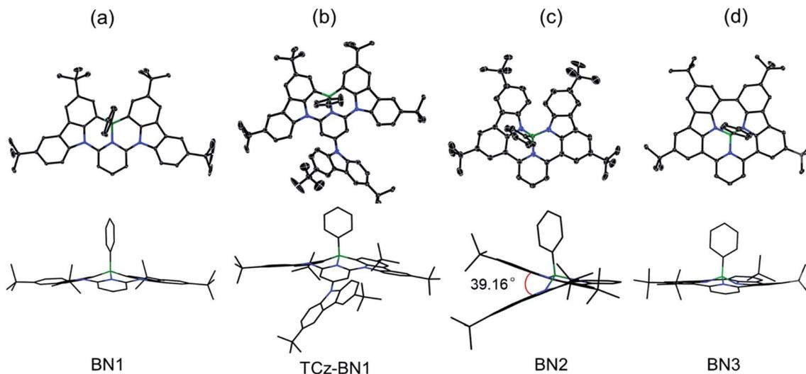
Fig. 2 X-ray crystal structures of (a) **BN1**, (b) **TCz-BN1**, (c) **BN2**, and (d) **BN3**, and the side views (bottom) of the structures in stick style. Hydrogen atoms and solvent molecules are omitted for clarity. The thermal ellipsoids are drawn at the 50% probability level.
