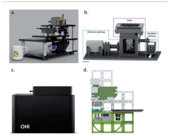
Fig. 6 (a) LiteTIRF microscope (reprinted from ref. 85), (b) miCube setup (reprinted from ref. 147), (c) ONI Nanoimager (reprinted from ref. 148), and (d) UC2 microscope (reprinted from ref. 153).
