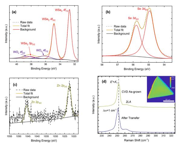
Fig. 2 XPS spectra reporting the individual core level spectra of W 4f (a), Se 3d (b) and Zn 2p (c). (d) Typical Raman spectrum of the as-grown WSe<sub>2</sub> monolayer and after PMMA-transfer on target SiO<sub>2</sub>. The principal  $E' + A'_1$  and 2LA peaks are indicated alongside their change after transfer. Inset: map of the  $E' + A'_1$  peak position of the CVD grown WSe<sub>2</sub> monolayer.
