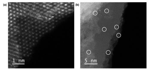
Fig. 4 Atomic scale ADF-STEM characterization of multilayered WSe<sub>2</sub>. (a) Micrograph of a monolayer portion of the WSe<sub>2</sub> flake where brighter spots suggest the presence of adatoms and (b) larger view of the distribution of adatoms on the WSe<sub>2</sub> plane.
