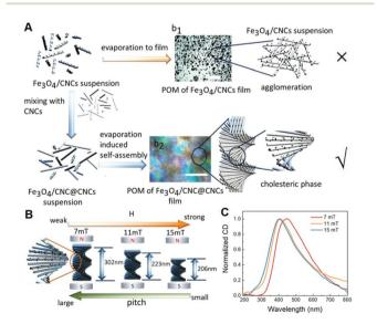
Fig. 4 (A) Synthetic scheme of self-assembly progress of chiral Fe $_3$ O $_4$ / CNC@CNCs films. (B) The relationship between the pitch of chiral structure and the applied magnetic field. (C) CD spectra for Fe $_3$ O $_4$ / CNC@CNCs films with different applied magnetic fields ranging from 7 to 15 mT. Adapted with permission from ref. 73. Copyright 2020, American Chemical Society.
