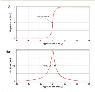
Fig. 2 (a) Langevin curve and (b) PSF for an ideal SPION
