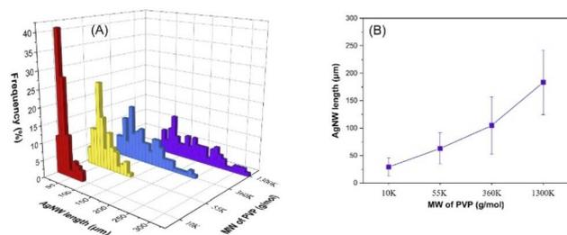
Fig. 4 Influence of PVP MW on the AgNW length distribution (A) and the average length of the nanowires (B).
