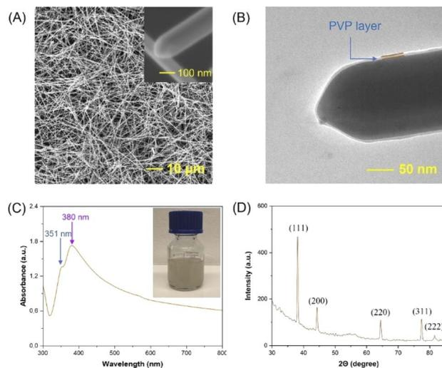
Fig. 1 SEM (A), TEM (B), UV-Vis (C) and XRR (D) characterization results of the AgNWs.
