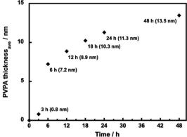
Fig. 2 The average thickness of PVPA in silica@PVPA with various PVPA polymerization times (12–48 h) determined by SEM observation.
