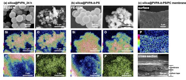
FE-SEM and SEM-EDX images of (a) silica@PVPA\_24 h, (b) silica@PVPA-b-PS, and (c) silica@PVPA-b-PS/PC membranes
