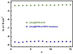
Fig. 7 (a) Humidity dependent proton conductivities and (b) repeated test of temperature- and RH-dependent proton conductivities of pelletized silica@PVPA\_24 h, silica@PVPA-b-PS, and silica@PVPA-b-PS/PC membranes.
