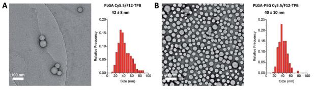
Fig. 2 TEM images (left) and corresponding size distribution histograms (right) for PLGA (A) and PLGA-PEG (B) NPs loaded with 20 mM Cy5.5/ F12-TPB dye. The values correspond to the average NP diameter, while errors correspond to the half-width at the half maximum. At least 200 NPs were analyzed per condition.
