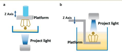
Fig. 1 Schematic illustration for the "bottom-up" (a) and "top-down" (b) printing technologies based on digital light processing (DLP) of photocurable materials.
