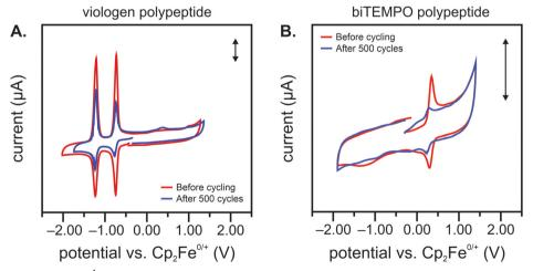
Fig. 5 Cyclic voltammetry at 100 mV s<sup>-1</sup> of the (A) viologen polypeptide anolyte and (B) biTEMPO polypeptide catholyte before and after cycling of the polypeptide redox flow cell (arrows denote 10 µA). Glassy carbon was used as the working electrode, platinum wire as the counter electrode, un-fritted freshly anodized Ag/AgCl wire as the reference electrode, and ferrocene was used as internal reference. The supporting electrolyte was 0.5 M TEATFSI in ACN.
