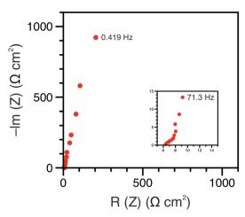
**Fig. 3** Nyquist plot of the EIS data before galvanostatic cycling for the redox flow cell with a BiTEMPO polypeptide catholyte and viologen polypeptide anolyte. EIS was conducted with circulating electrolytes at open circuit potential with an amplitude of 10 mV in a frequency range of 200 kHz to 0.4 Hz (5 steps per decade).
