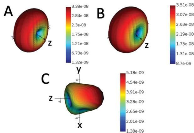
**Fig. 4** Calculated far-field profiles of the gold nanorod dimer-1. (A) Dimer excited by LCP light at the anti-bonding wavelength of 709 nm, and at the bonding wavelength of 774 nm (B). (C) Off-resonance excitation at 650 nm of the gold nanorod dimer.
