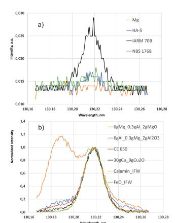
Fig. 5 Line scans around 130.22 nm (700 V, 20 mA). (a) Intensities of the pure compact samples. (b) Normalized intensities of selected samples with high oxygen concentration.
