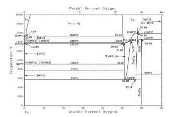
Fig. 2 Assessed Fe-O phase diagram, Condensed system 0.1 MPa, Copyright (C) 1996 ASM International.
