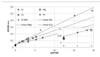
Fig. 4 Calibration curves for 130 nm with all samples.
