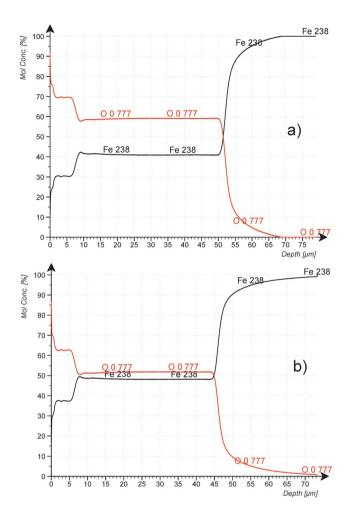
Fig. 8 CDP analysis of construction steel oxidized at 800 °C for 10 min at 200 mbar  $O_2$ . (a) using the emission yield of the calibration in Fig. 6 and (b) using the emission yield of FeO\_IFW.
