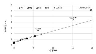
Fig. 6 Calibration curve for 777 nm including all calibration samples (measured by a Peltier cooled PMT and monochromator).
