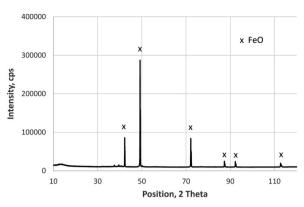
Fig. 3 XRD measurement (Co K $\alpha$  radiation) on the backside of the layer grown in 10 min on construction steel at 800 °C and 200 mbar O<sub>2</sub>.
