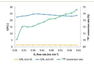
Fig. 1 Evaluation of the oxygen flow rate in CRC, based on S/N in the case of m/z equal to 31 (orange line) and 47 (blue line), and the estimation of the  $^{31}P^{+}$  to  $^{31}P^{16}O^{+}$  conversion rate (green line).
