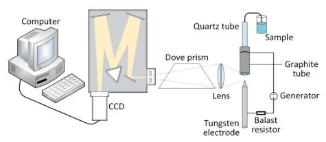
Fig. 1 A schematic representation of the HDC-APGD-DP-OES experimental system.
