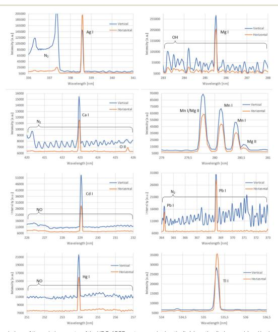
Fig. 6 The morphology of the emission spectra of the HDC-APGD system acquired vertically (along the discharge axis) and horizontally (with the use of the Dove prism) in the vicinity of the analytical lines of Ag, Ca, Cd, Hg, Mg, Mn, Pb and Tl.
