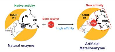
Fig. 1 Schematic representation of the design of ArMs: left, the natural catalysis in TbADH WT involving NADP $^+$  and a catalytic Zn $^{2+}$ ; right, the supramolecular insertion of an iridium piano stool complex (red) inside the NADP $^+$  cofactor pocket and Zn $^{2+}$  binding region of TbADH 5M with high affinity induced by the anchor substructure (R).
