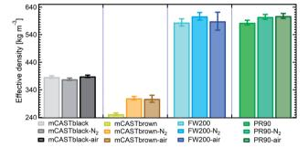
Fig. 18 The effective density ( $\rho_{\rm eff}$ ) of fresh and denuded 200 nm soot particles. The error bar indicates one standard deviation. Please note the y-axis origin.
