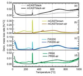
Fig. 17 TGA derivative mass loss rates as a function of temperature (T) for fresh and synthetic air ( $N_2 + O_2$ ) atmosphere oven heated (300 °C) bulk soot samples solid and dotted lines indicate two individual TGA runs on the same sample type.
