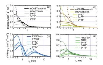
Fig. 8 The pore size distribution (PSD) as a function of pore radius  $(r_{\rm p})$  for fresh and synthetic air  $(N_2+O_2)$  oven-heated soot with different contact angle assumptions, derived from DVS isotherms shown in Fig. 7. (a) mCASTblack, (b) mCASTbrown, (c) FW200, (d) PR90. In each panel, solid line, dotted line and dashed line indicate the PSD results of the same soot sample with different soot–water contact angle assumption values.
