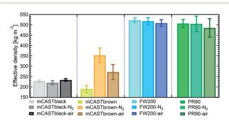
Fig. 6 The effective density ( $\rho_{\rm eff}$ ) of fresh and denuded 400 nm soot particles. The error bar indicates one standard deviation. Please note the y-axis origin.
