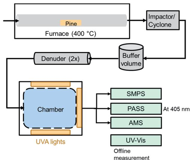
Fig. 1 Experimental setup for the generation, aging and detection of BrC photoreaction. UV-vis was used as an offline technique and required a separate experiment to the online techniques. The AMS was not used for every experiment. The denuders were composed of activated charcoal. The UVA lights were centered at approximately 360 nm (see Fig. S1†). SMPS: scanning mobility particle sizer. PASS: photoacoustic soot spectrometer. AMS: aerosol mass spectrometer.
