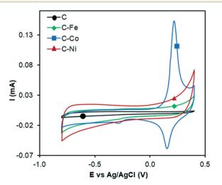
Fig. 6 Cyclic voltammograms in  $N_2$ -saturated KOH solution at 1000 rpm and 50 mV s<sup>-1</sup> of C, C–Fe, C–Co and C–Ni.
