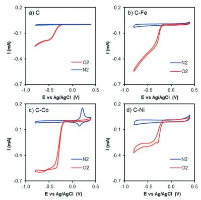
Fig. 7 Cyclic voltammograms at 1000 rpm and 50 mV s<sup>-1</sup> of a) C, b) C-Fe, c) C-Co and d) C-Ni with N<sub>2</sub> bubbling (blue line) and O<sub>2</sub> bubbling (red line) in KOH solution.
