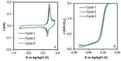
Fig. 9 Reuse tests of the C-Co sample. a) Cyclic voltammograms at 1000 rpm and 50 mV s<sup>-1</sup> and b) LSV curves at 1000 rpm and 5 mV s<sup>-1</sup>.
