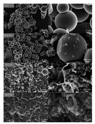
Fig. 1 SEM images of pure (C) and doped (C-Fe, C-Co and C-Ni) samples obtained by LDPE pyrolysis.
