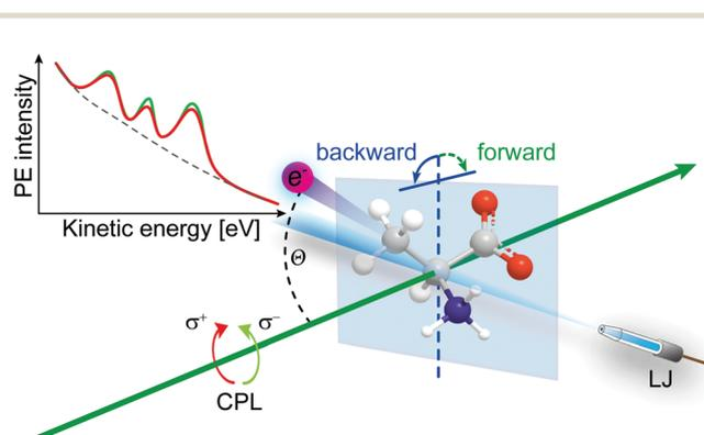
Fig. 7 Depiction of the liquid-jet PECD experiment with backward electron detection relative to the light propagation (green arrow); CPL denotes circularly polarized light. Inset: Fictive carbon 1s PECD spectrum on top of the LET. Illustrated intensity differences correspond to measurements with left- and right-CPL from the same enantiomer in water.
