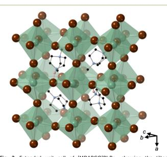
Fig. 2 Extended unit cell of [MDABCO]RbBr3, showing the tilted orientations of four MDABCO dications within the pseudo-cubic framework of corner-sharing RbBr<sub>6</sub> octahedra. C, N, Rb and Br are shown in black, blue, green and brown, respectively. H atoms are omitted for clarity, apart from N-H atoms (pink) involved in hydrogen bonds, which are indicated by dashed red lines.
