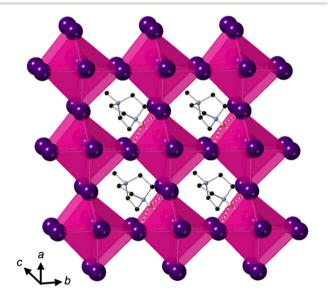
Fig. 1 Four adjacent pseudo-cubic motifs of [MDABCO]CsI<sub>3</sub>, showing alignment of the MDABCO N-N axes along the unique axis (c). C, N, Cs and I are shown in black, blue, pink and purple, respectively. H atoms are omitted for clarity, apart from N-H atoms (pink) involved in hydrogen bonds, which are indicated by dashed red lines.
