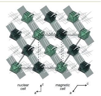
Fig. 4 Magnetic structure of  $Cr[Bi(SCN)_6] \cdot xH_2O$ . Magnetic Cr atoms are coloured in green and black to illustrate their relative orientations, and the other non-magnetic framework atoms are shown in grey. The  $\{111\}_{cubic}$  type planes in which all spins are ferromagnetically correlated are highlighted. The magnetic and nuclear unit cells are related as follows:  $a_{mag} = a_{nuc} - c_{nuc}$ ,  $b_{mag} = -b_{nuc}$  and  $c_{mag} = -2a_{nuc}$ .
