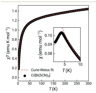
Fig. 2 Variable temperature magnetic susceptibility product measured over the range 2-300 K (zero field cooled). Inset shows the magnetic susceptibility measured over 2-10 K, highlighting magnetic order. Orange dashes line indicates the Curie-Weiss fit, carried out over the range 20 to 300 K.
