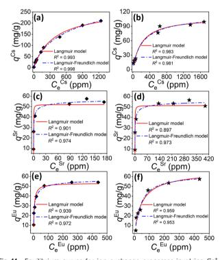
Fig. 11 Equilibrium curves for ion exchange processes involving Cs<sup>+</sup> (a and b),  $Sr^{2+}$  (c and d), and  $Eu^{3+}$  (e and f) using compounds H<sub>2</sub>O. The red lines and dotted blue lines represent fitting of the data with Langmuir and Langmuir-Freundlich isotherm models, respectively. The images in (a-f) were reproduced form ref. 135 with permission form ACS, copyright 2021.
