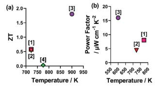
Fig. 7 Figure showing the reported zT and power factor (PF) values for non-oxide HE metal chalcogenides. Where [1] Cu5Sn1.2MgGeZnS9, [2], (CoFeNi)(SSe), [3] (PbSbSn)(SSeTe), [4] (AgPbBi)(SSeTe) correspond to ref. 37, 47, 54 and 66.
