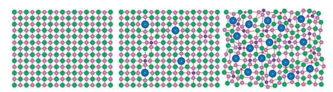
Fig. 4 Figure visually showing the distortion in the lattice structure of a (PbSbSn)(SSeTe) HEMC where the pink, red, green, blue, and purple spheres represent Pb, Sn, Se, Te, and S atoms, respectively. Copyright permission from Science, used from ref. 37.
