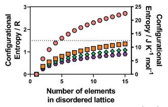
Fig. 1 Calculated configurational entropy (in both R and J K<sup>-1</sup> mol<sup>-1</sup>) for species with a single disordered sub-lattice (M) for (pink circles) alloys with a single lattice, and a range of common metal chalcogenide materials with a single chalcogenide sub-lattice (i.e. X is all O, S, Se or Te) for (orange squares) MX, (blue diamonds) M<sub>2</sub>X<sub>3</sub> and (purple hexagons) MX<sub>2</sub>.
