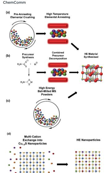
Fig. 3 Figure showing a schematic representation of extant synthetic procedures toward high entropy metal chalcogenides. (a) elemental annealing (b) thermolysis of single source precursor cocktails (c) high energy ball-milling of individual metal sulphides (d) nanoparticle cation exchange.
