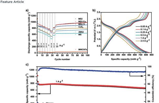
Fig. 6 (a) Galvanostatic rate performance test of all HESs, CoS<sub>2</sub>, 4MS2, and MWCNTs half-cell at different current densities and 25 °C in the voltage range between 0.01 and 3 V versus Li<sup>+</sup>/Li. (b) Voltage profiles of MS2 half-cell at different currents. (c) Specific charge/discharge capacity of MS<sub>2</sub> half-cell and Coulombic efficiency as a function of cycle number at 1 C and 25 °C in the range between 0.01 and 3 V. Copyright permission from Wiley, used from ref. 52
