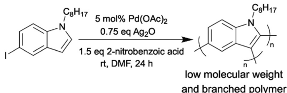
Scheme 10 Room-temperature DARP of 5-iodo-1-octylindole monomer.
