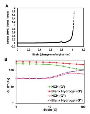
Fig. 7 Mechanical properties of the hydrogels. (A) Compressive stressstrain curves for the NCH system with the load endpoint set at 50 N. (B) Storage (G') and loss (G'') moduli obtained using dynamic frequency sweep test from 0.1 to 100 rad s<sup>-1</sup>.
