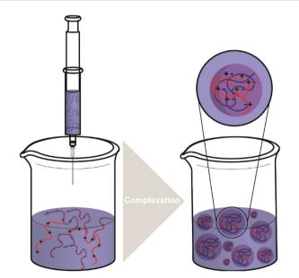
Scheme 4 The typical processes of forming polysaccharide NPs such as CS/HA NPs by complex coacervation process.
