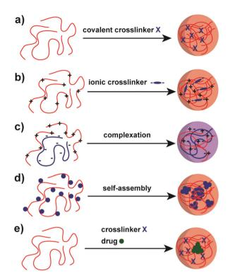
Scheme 2 Avenues for the preparation of polysaccharide NPs: (a) covalent crosslinking, (b) ionic crosslinking, (c) complexation of oppositely charged polysaccharides, (d) self-assembly of hydrophobically (blue sphere) modified polysaccharides and (e) polysaccharide-drug (green sphere) conjugate.<sup>25</sup>
