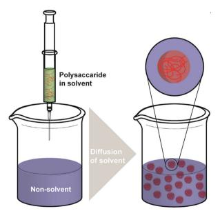
Scheme 3 Schematic representation of the nanoprecipitation method.
