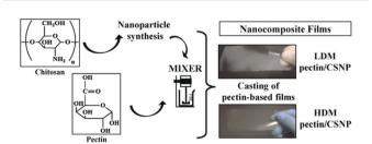
Fig. 15 Overview of nanocomposite formation from pectin and CS NPs and casted films. (Reproduced with permission from ref. 282. Copyright
