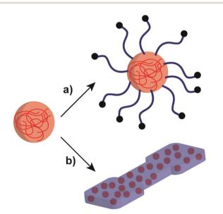
Scheme 6 Schematic representation of the polysaccharide NP incorporation with polymer systems: (a) polymer-grafted polysaccharide NP and (b) polysaccharide NPs in a polymer matrix
