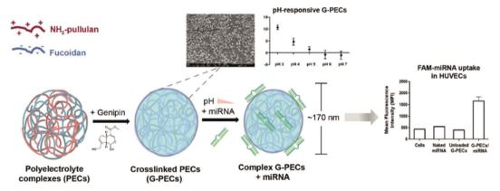
Fig. 11 Formation of  $NH_2$ -PL/fucoidan coacervate NPs and loading with microRNA (miRNA) (left), particle characterisation via SEM and pH response (top) and mean fluorescence intensity (MFI) of fluorescein amidite (FAM) measured by flow cytometry analysis revealing the uptake in human umbilical vein endothelial cells (HUVECs) (right). (Reproduced with permission from ref. 236. Copyright Elsevier, 2021.)
