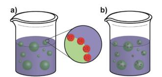
**Scheme 8** (a) Structure of a polysaccharide NP stabilised Pickering emulsion and (b) Pickering emulsion with cargo loaded droplets.
