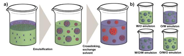
Scheme 5 Schematic overview over the emulsion process for polysaccharide NP formation: (a) formation of polysaccharide NPs via water-in-oil emulsion and crosslinking (external gelation) and (b) types of emulsions used to prepare polysaccharide NPs (green: organic solvent; blue: water).
