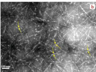
Fig. 2 (a and b) TEM images of cellulose nanofiber dispersion after TEMPO-mediated oxidation and ultra-sonication. The fibers are highlighted by yellow
