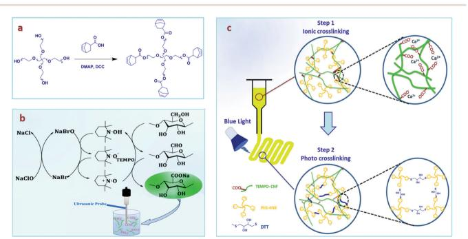
Fig. 1 Schematic for: (a) synthesis of 4-arm poly(ethylene glycol)-norbornene (4PEG-NB), (b) synthesis of cellulose nanofibers (CNFs) via TEMPO-mediated oxidation and high energy ultrasonication treatment, and (c) 3D bioprinting process via the dual mode crosslinking of the PEG-CNF ink. Dual crosslinking system: physical (ionic crosslinking, step 1) + chemical crosslinking (photo crosslinking, step 2).
