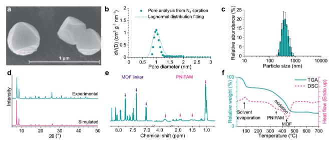
Fig. 2 Characterization of UiO-66-PNIPAM in terms of morphology and chemistry via (a) SEM, (b) nitrogen sorption, (c) DLS, (d) XRD, (e) NMR, and (f) DSC-TGA. Details of the characterization methods and the results for the other five MOFs are presented in the ESI.
