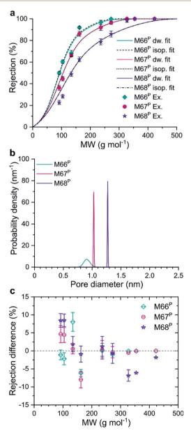
Fig. 5 (a) Experimental rejections and fitted MWCO curves assuming log-normal pore size distribution (PSD) or isoporosity. (b) Log-normal PSDs of the membranes obtained from the fitting. (c) Rejection difference between the isoporous fit and experimental data points.
